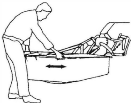
Fig. 8. Supporting mower when removing transport beam.
