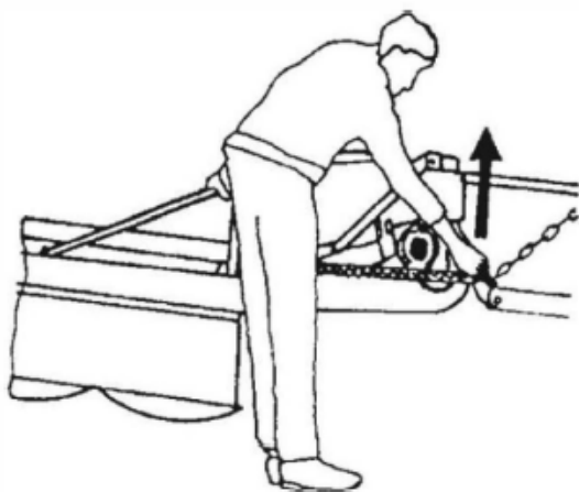
Fig. 8. Supporting mower when removing beam.
